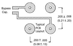
An External 0.01uF Bypass Capacitor is required between VDD and GND.
