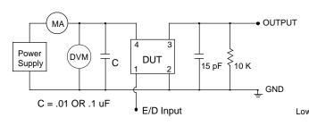
**E/D (Enable/Disable)** Input has an internal pull-up resistor. It can be left floating or connected to Vdd.
