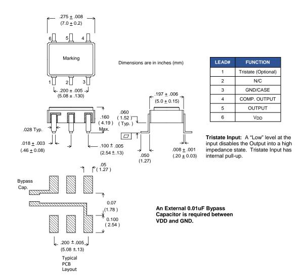
Figure 1 - Package Configuration & Pin Connections
