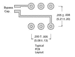
An External 0.01uF Bypass Capacitor is required between VDD and GND.
